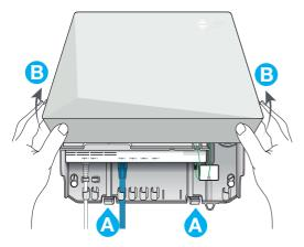
Press the two clips **A** to release the cover. Lift the cover at an angle to remove **B**.
