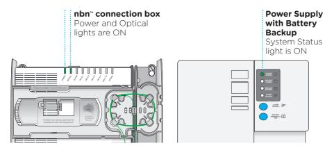
If you remove the cover from your **nbn**™ connection box and the lights on your **nbn**™ connection box or Power Supply with Battery Backup (if installed) do not match those shown in this diagram, then refer to the lights and indicators sections of this guide on pages 14–15 and 25.
